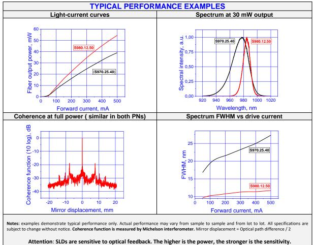
All parameters are measured at optical feedback not exceeding 1E-3.
